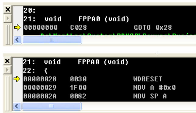
Fig. 6: Stack Assignment in Mini-C project
